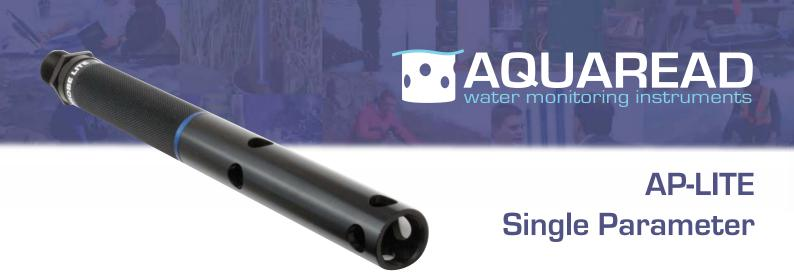
The AP-LITE is a simple probe with a single optical socket. This socket is able to house any of our optical electrodes, including turbidity and chlorophyll. A temperature sensor is also included on the probe. The AP-LITE package includes our rugged 3m cable, our GPS Aguameter, a range of accessories and a rugged carry case.
